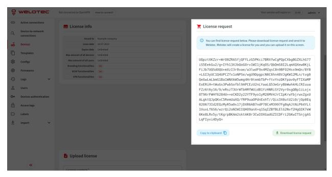
License request will be shown. You can copy it to a clipboard or download it to a file. Please send generated license request to Welotec so we can generate an appropriate license for you. The generated license should be uploaded to the system using the "Upload license" form.
